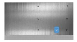
along the backwall, C and D were on the horizontal midline, and E and F were along the front intake grate. A, C, and E were placed on the front to back center line, and B, D, and F were 6" off the sidewall.
